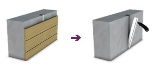
After pouring of concrete & removal of the shuttering, remove the polystyrene infill using a knife to cut through the two continuous groves in the infill. Remove the nails.
