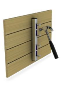
Fix the Concrete Insert to the shuttering by nailing through the slots created by the anchor lugs. Fit end caps as necessary to the open ends of the concrete insert. The anchor lugs can be wired onto reinforcement mesh as required to increase the strength of the finished assembly.
